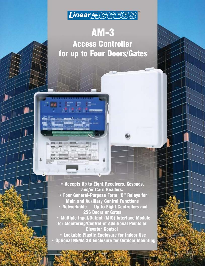
The AM-3 Multi-portal access controller has four built-in General purpose (form "C" relays). Each can be configured for open/close. Any one can be used for the control relay and the others for a myriad of auxiliary control functions, including activation of safety edge reverse, external lighting, or alarm shunting. In addition, the AM-3 supports request to exit and door status monitoring for each relay. All relay contacts have extensive RFI, ARC, and lightning suppression.
